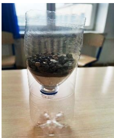
Figure 1. Independently constructed filtration device
