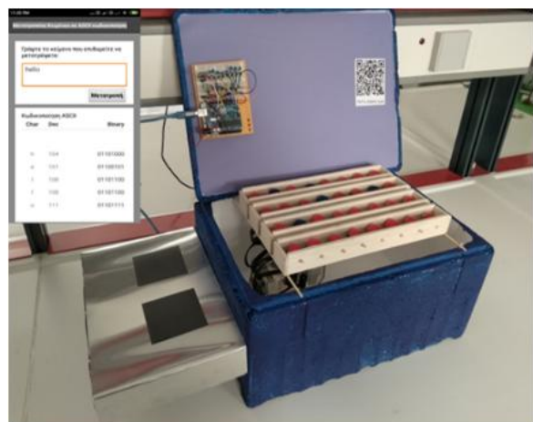
Picture 4. The flash-memory drive model based on spintronics
